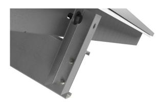
**PIVOT ADAPTER** The uniquely designed pivot adapter elevates each one-point purlin connection to drastically improve every table's adaptability to challenging topography. The fully grounded rows can adjust to changes up to 20% grade.
