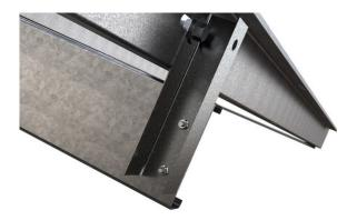
INTEGRATED BONDING Each continuous row is bonded using serrated hardware, therefore only one ground is needed per row. No additional costly grounding components needed such as WEEBS and star washers, lowering material and installation costs. This reduces labor time, hardware, and cost for additional bonding components. (Certified to UL 2703)
